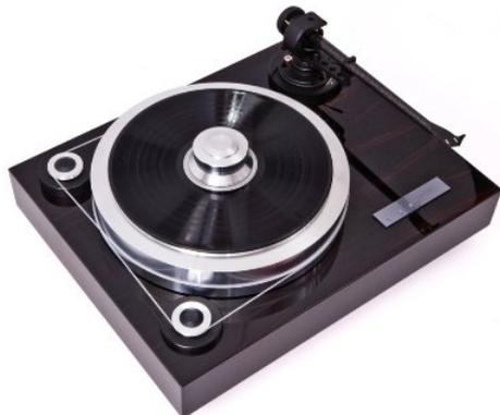
As to the bearing, EAT Forte S employs an inverted construction in which the platter (the Teflon cup) rests on a ceramic ball on the top of a pin. In order to reduce the pressure on the ceramic ball from becoming too heavy, two enormous neodymium magnets hold the platter 'in the air'.
