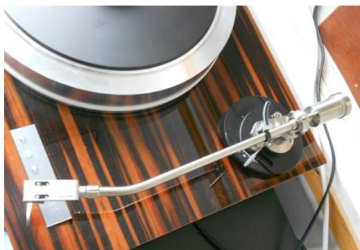
The EAT-312 has no anti-skating adjustment, or rather, preadjusted anti-skating is in-built. That's sufficient for majority of cartridges that go with it, such as heavy Ortofon SPUs but also for somewhat lighter carts. When the tracking force is beyond 2,5 grams, it's arguable that anti-skating loses its importance.
