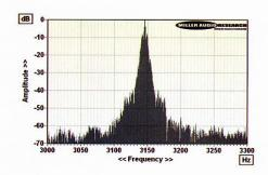
ABOVE: Wow and flutter re. 3150Hz tone at 5cm/ sec (plotted  $\pm 150$ Hz, 5Hz per minor division). Wow is very low and flutter, though complex, is also low
