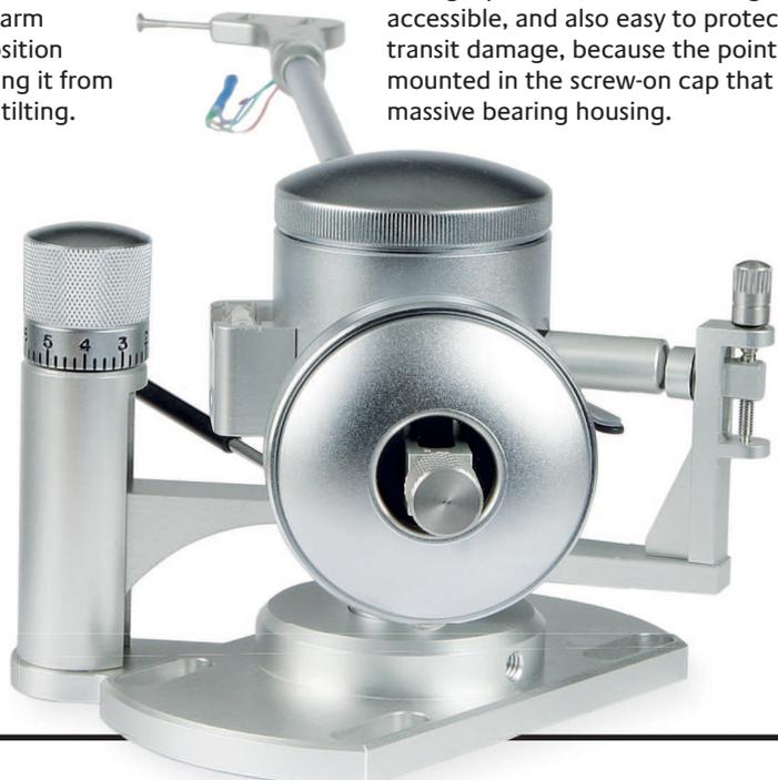
**RIGHT:** Seen far right is the Magneglide stabiliser, using magnets in line with the arm's pivot point. The outrigger magnet can be moved up or down for azimuth correction
