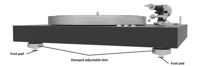
Three precision adjustable damped feet are mounted under the turntable for leveling the turntable. Once the turntable is in final position, put the supplied spirit level on the chassis and then level the turntable by screwing or unscrewing the feet as needed. It is advisable to check level from several positions on the chassis.
