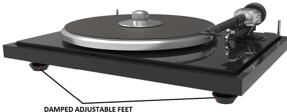
Three precision adjustable damped feet are mounted under the turntable for leveling the turntable. Once the turntable is in final position, put the supplied spirit level on the sub-chassis, and then level the turntable by screwing or unscrewing the feet as needed. It is advisable to check level from several positions on the subchassis.
